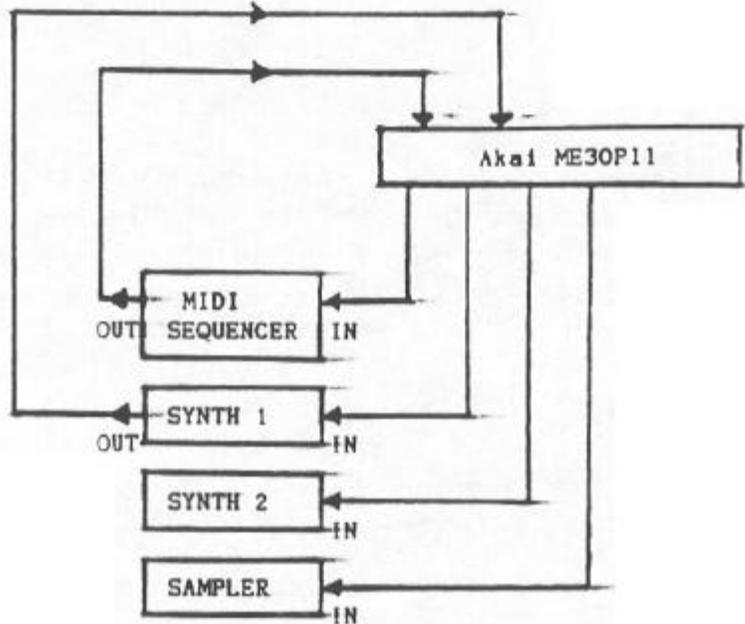
FIG. 2b Connecting a MIDI sequences to MIDI synths using the Akai ME30PI1
