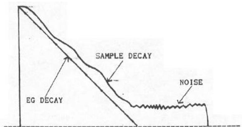
Fig. 1 Fading out noise using the envelope generators
