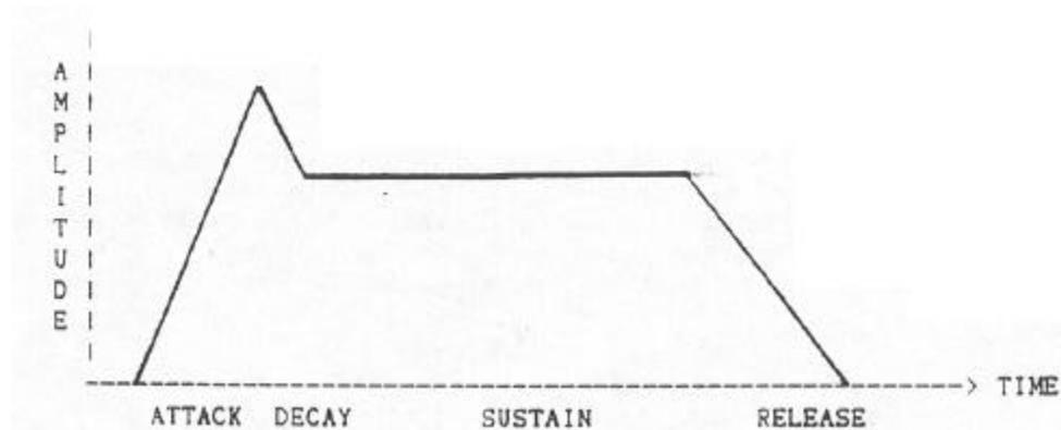
Furthermore, most, if not all acoustic instruments exhibit tonal envelope changes where the tone varies during the course of a note. By providing a separate envelope generator for the filter, we are also able to imitate these effects as well as set up some interesting, electronic effects.
