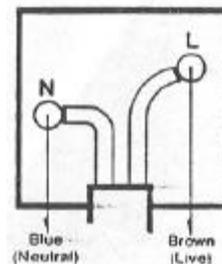
Do not connect any wire to the larger pin marked E or down when wiring a plug. Ensure that all terminals are securely tightened and that no loose strands of wire exist.
